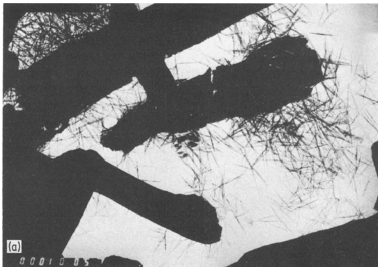
Figure 9 As-received plaster. (a) micrograph crystals; (b) selected area diffraction pattern.
