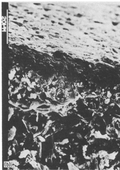
Figure 3 Composite figure showing the size and distribution of CSD at the surface after casting against glass and the concentration of potassium at the surface. ··· Analysis of surface; — analysis of section. The accelerating voltage is 30 keV and the take-off angle 45°.
